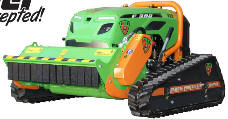
systems of maintaining slopes with hand-held line trimmers, and one of these mowers can do the work of ten operators, thus resulting in lower operative costs. The result is increased productivity with reduced liability.
